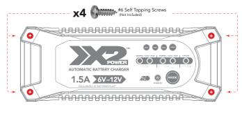
The SI C10003A has four (4) external holes for mounting. Mount the charger in a desired location with #6 self-drill screws. Make sure there are no obstructions behind the mounting surface. The DC cable length from the charger. with the clamp or eyelet, is approximately 23-inches (584.2mm). Allow for 12-inches (340mm) of slack between connections.
