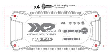
The SI C10005A has four (4) external holes for mounting. Mount the charger in a desired location with #6 self-drill screws. Make sure there are no obstructions behind the mounting surface. The DC cable length from the charger. with the clamp or evelet, is approximately 23-inches (584.2mm). Allow for 12-inches (340mm) of slack between connections.
